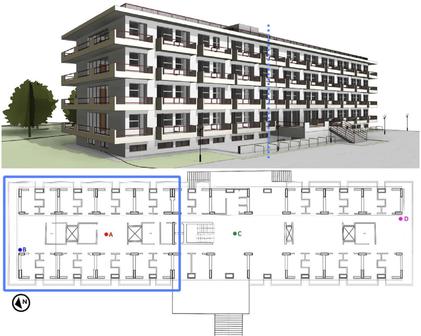
Fig. 1. Ground floor plan of the Athens case study. In the blue box, separated by the expansion joint, the northern part of the building, and the different measuring stations.
