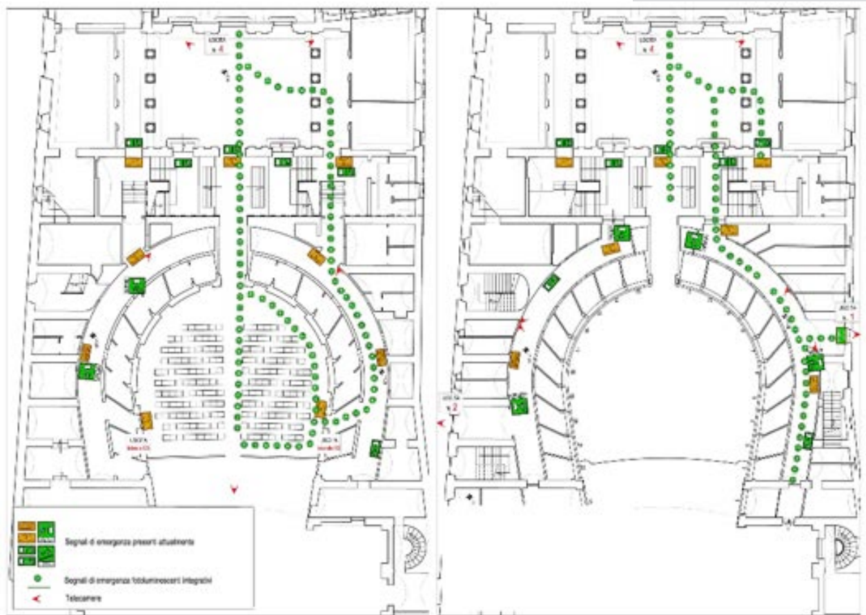
Figure 3. Application (position) of PS (right side of the theatre) and CS (left side of the theatre) during the evacuation drill.
