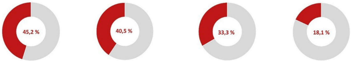
Fig. 3. Diagrams with the percentage of recovered material from the previous church for the roof's construction. From left (in red): recovery of arched ceilings, recovery of timber and slates for the roof, recovery of wooden floor frames and underlying ceiling, recovery of the lateral part coverage.
