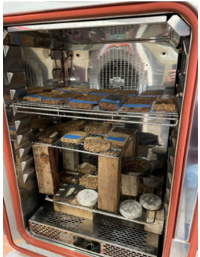
Fig. 2. Climatic chamber used for durability test.
