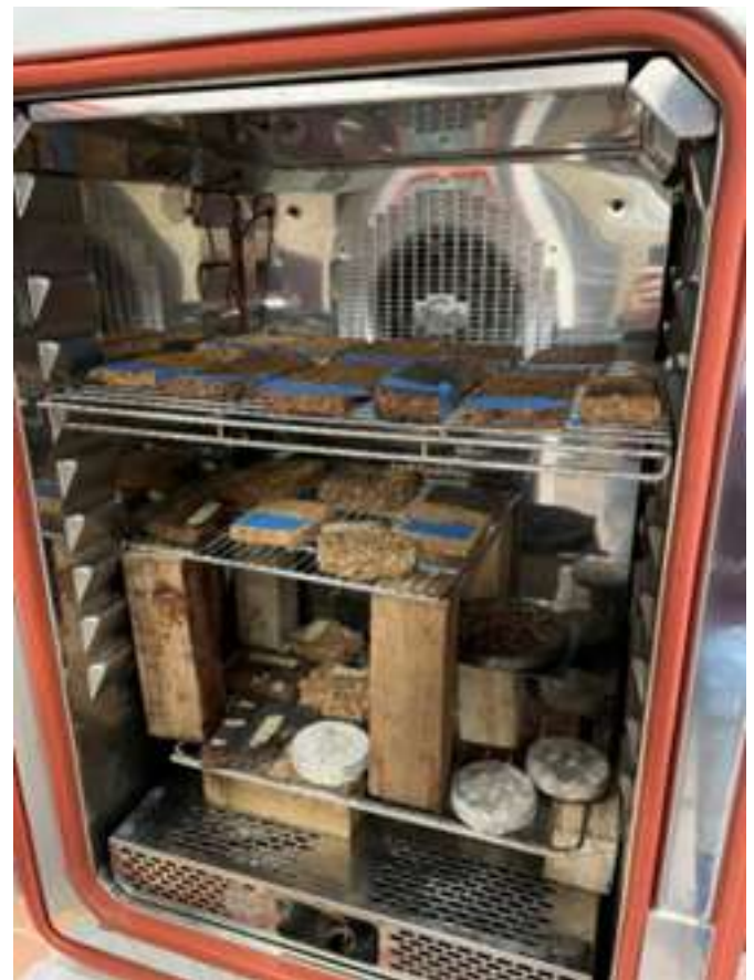
Fig. 2. Climatic chamber used for durability test.
