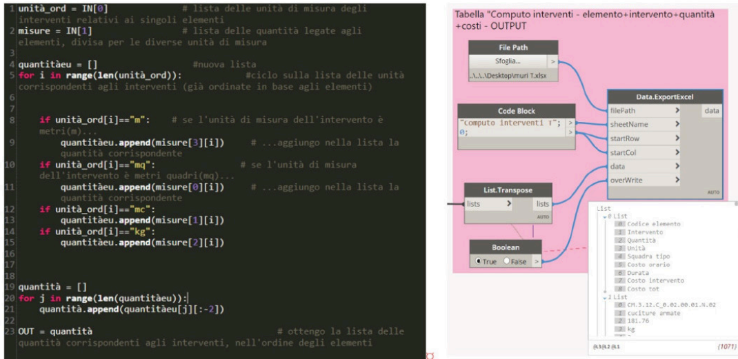
Fig. 4. On the left is an excerpt of the script that enables the relationship between tasks and the quantities of raw material related to the building object included in the task; on the right is the Dynamo node that manages the 'task/building object/quantities/costs' *.xls output, to be transferred by the orchestrator to the subsequent process phases.
