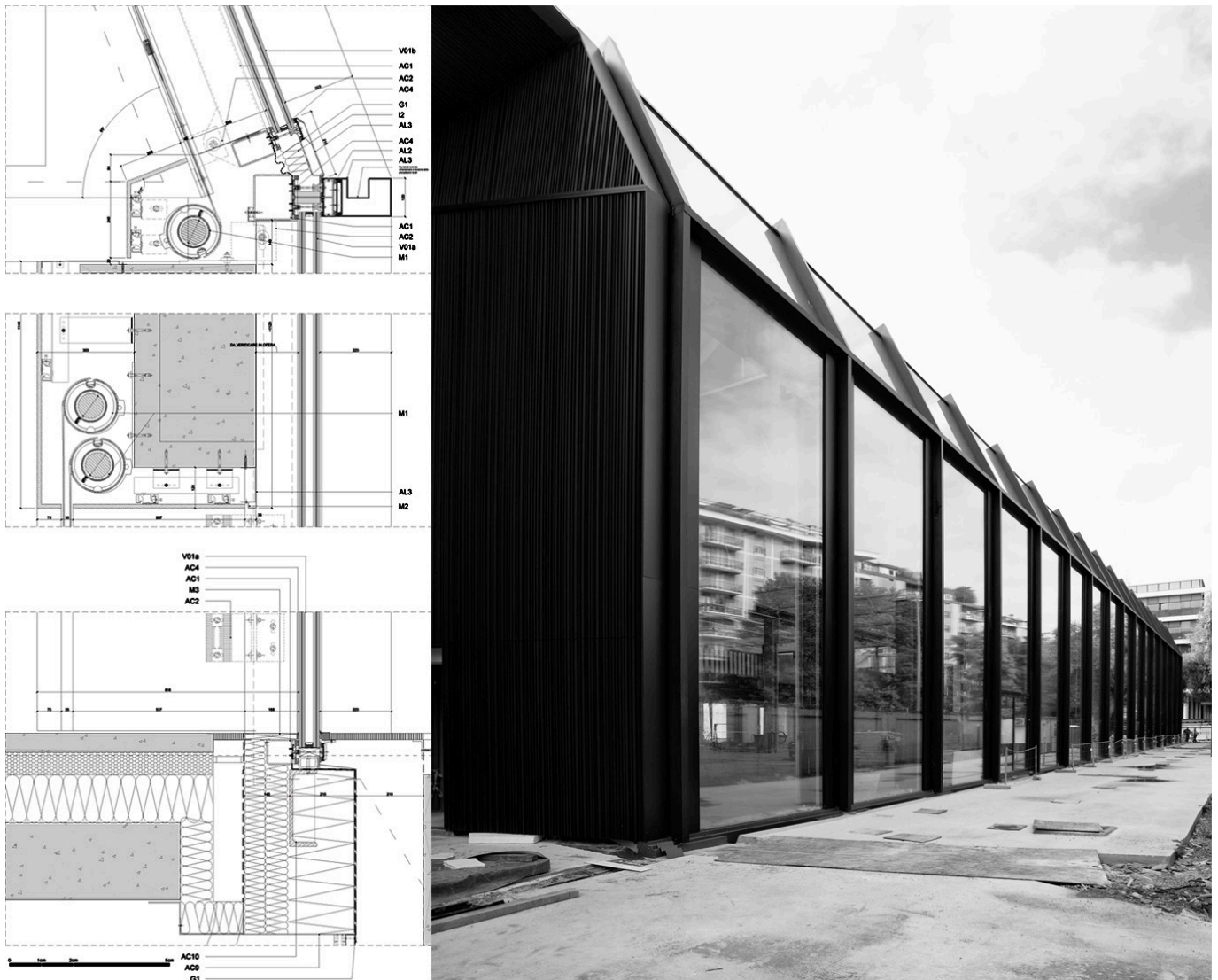
Fig. 4. The transparent façade on Via Tortona with the upper part shaped as the backward roof of the previous industrial building. Source: © Park Associati.
