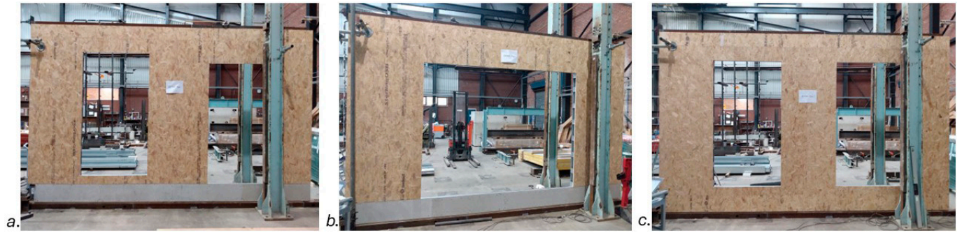
Fig. 5. Test rig of the walls with openings: (a) ground floor with 2 openings (GF-FW); (b) ground floor with one large door (GF-RW); (c) first floor (FF-FW) with two openings.
