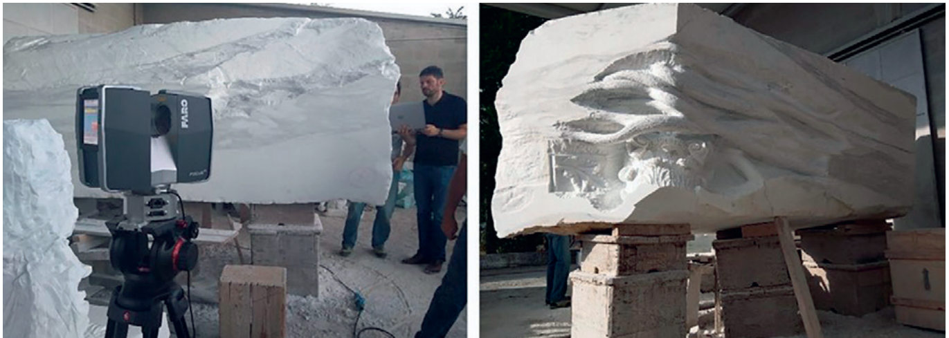
Fig. 4. 3D scanning of the 11,4 tons block of marble carved in the workshop of the stonemason.
