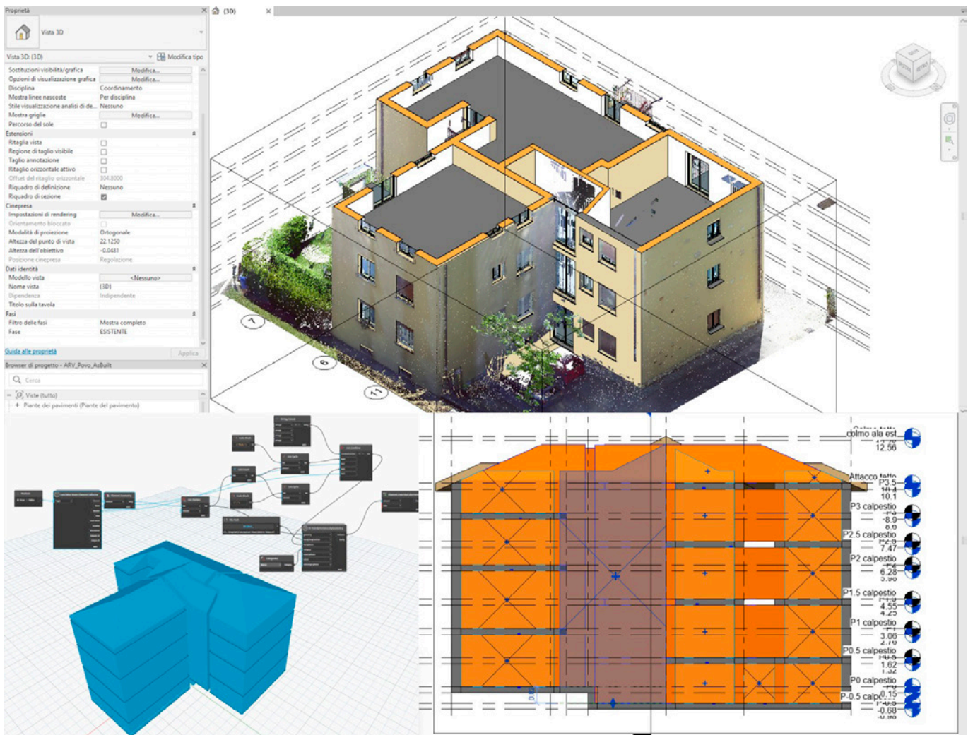
Fig. 10. The point cloud of the case study overlapped with the 3D model in the BIM environment. 3D and 2D visualisation of rooms allow for verifying proper separation between spaces before import in energy analysis software. Source: © 2023, the research group.
