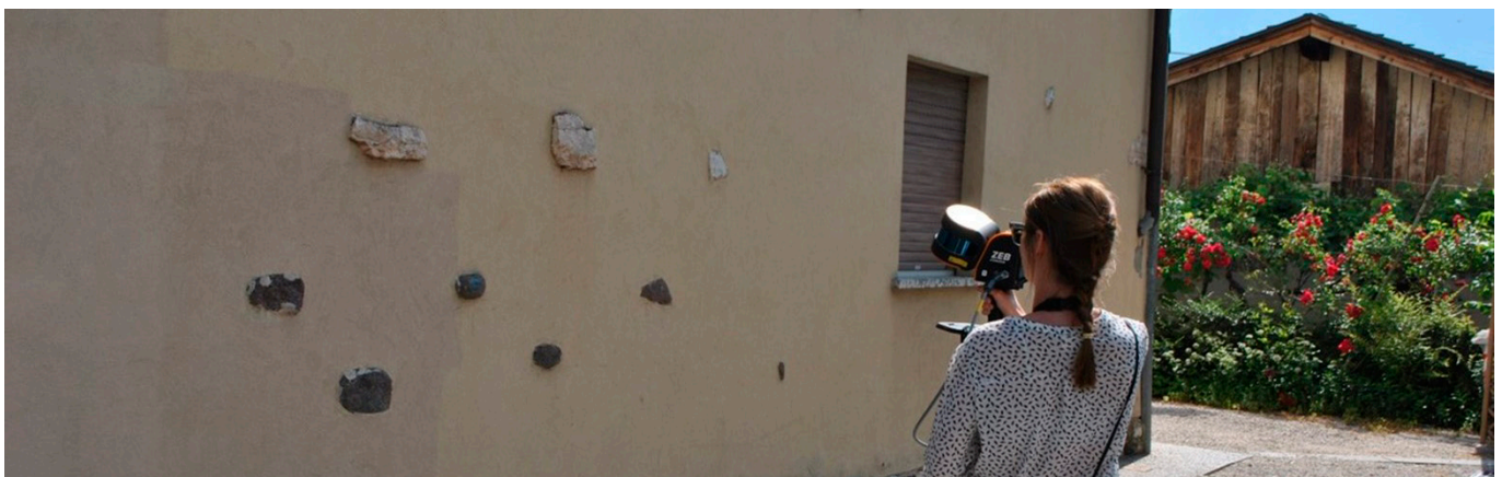
Fig. 6. The acquisition phase of the north façade with GeoSLAM Zeb Horizon from the ground floor photos. Source: © 2023, the research group.
