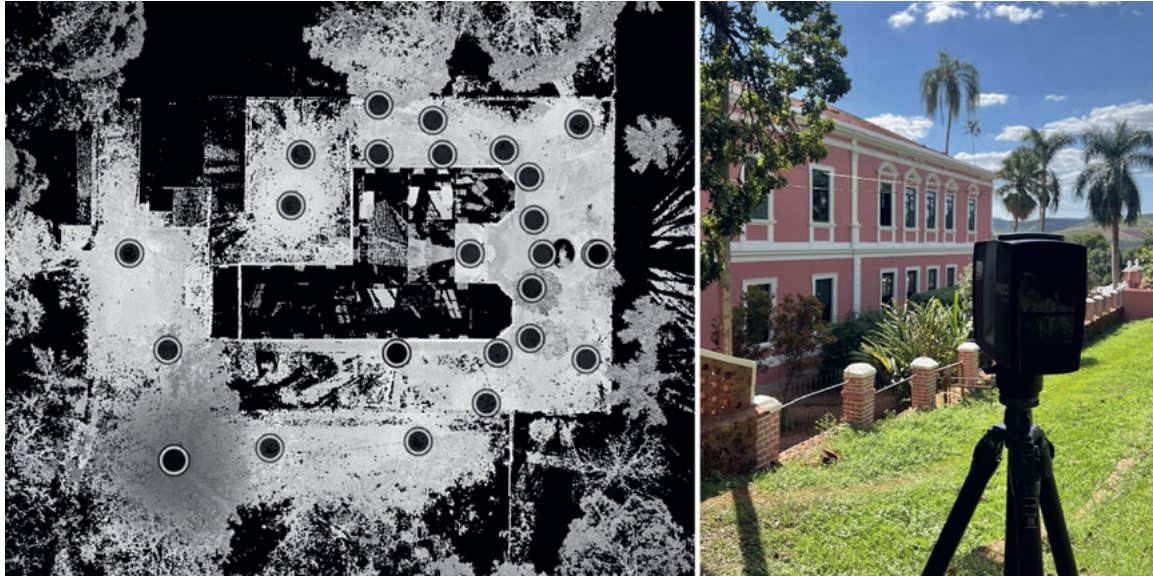
Fig. 8. Laser scanning process. Source: Authors.
