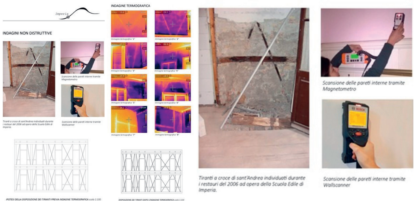
Fig. 5. Villa Ida. Non-destructive investigations to understand the structure: magnetometer survey and thermographic survey. Source: [7].
