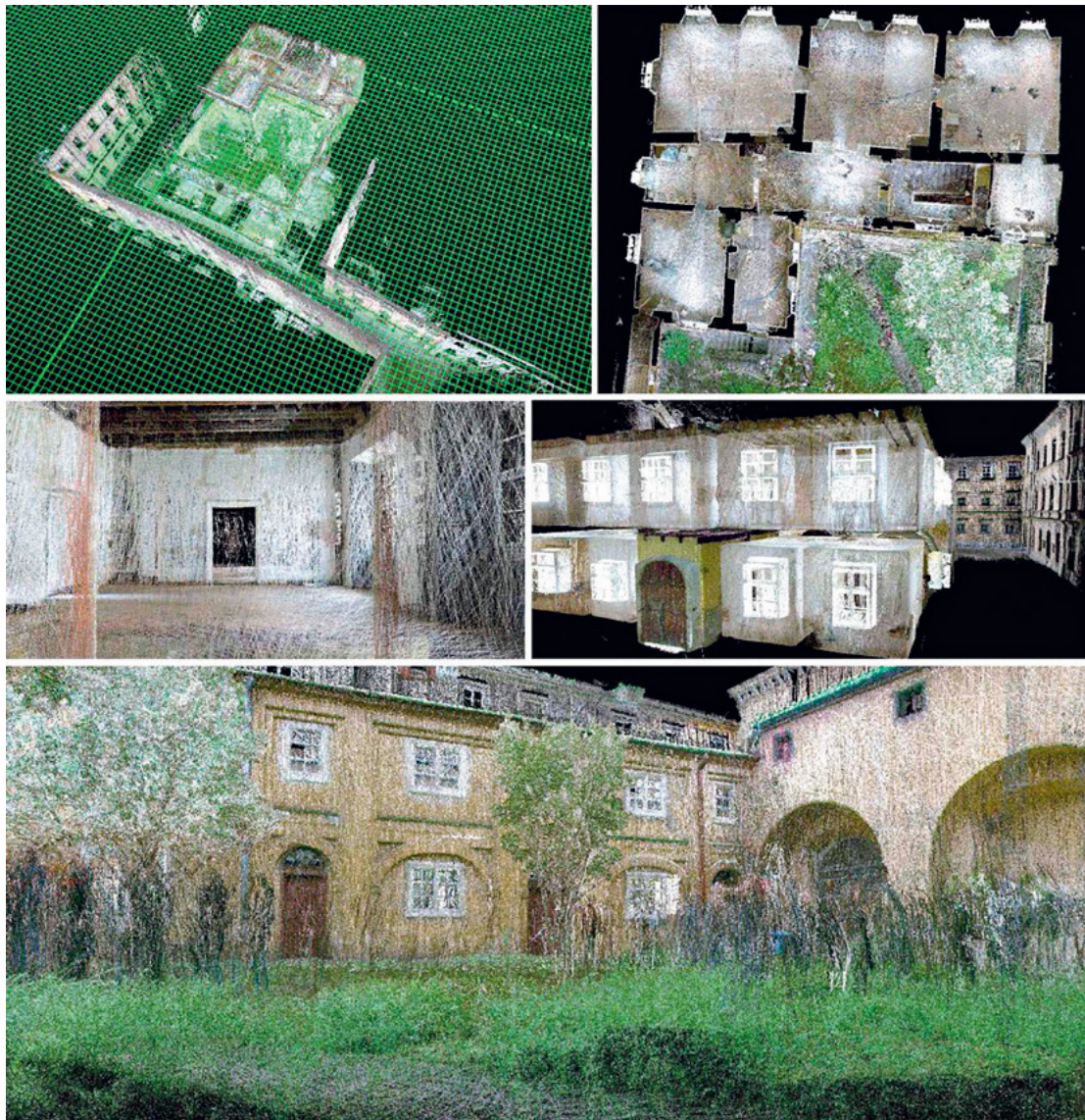
Fig. 3. Point cloud of BLK2GO Leyca Geosystem of the entire complex and inner garden. The acquisitions were realized following five different paths and registered together via Cyclone Register 360 software. Source: CC-BY SA [La Placa, 2024]; © 2025, Authors.
