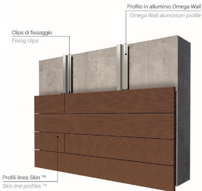
Fig. 5. Façade cladding panels schemes: (left) with an empty space between panels and the existing structure, for ventilation and (right) with insulation. © 2025, Iperwood®.
